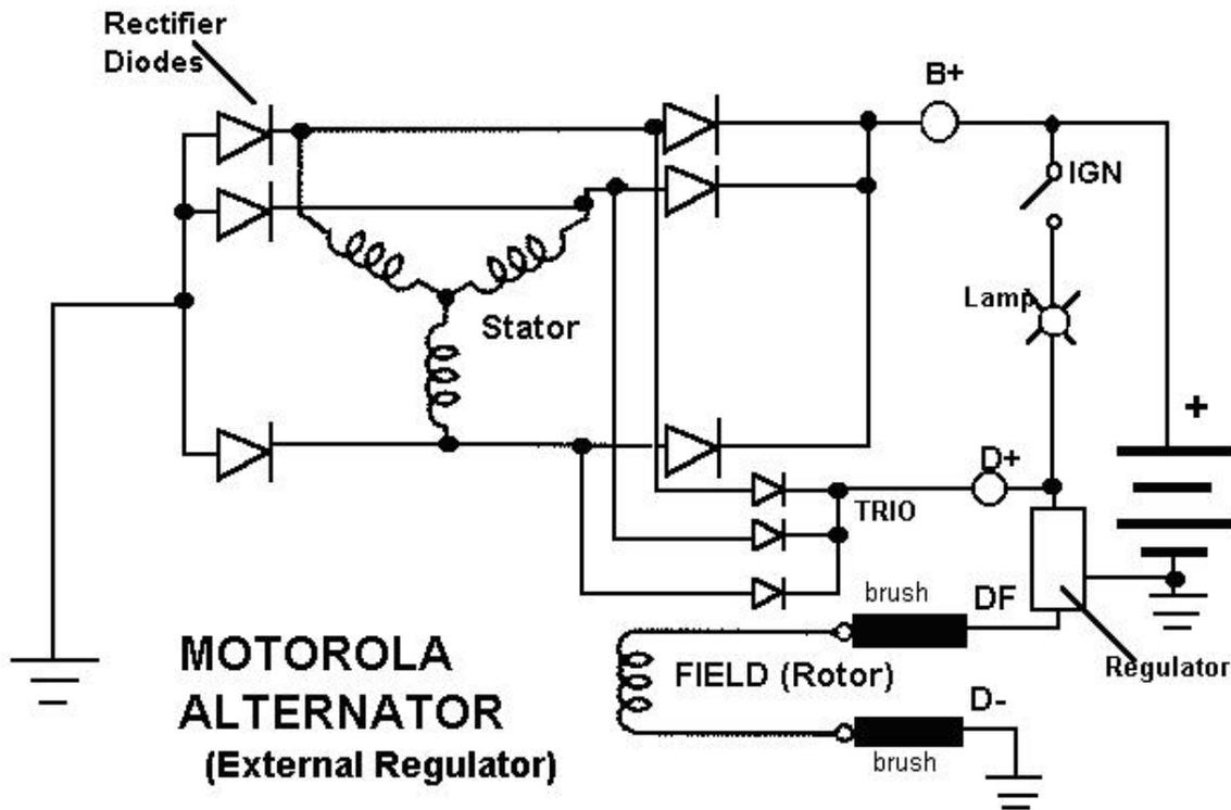
**Introduction** - The diagram above shows the internal wiring of the Motorola alternator with the external regulator. Generally all alternators generate a full wave rectified three phase output and use the battery as a smoothing device to produce the DC voltage we are familiar with.
